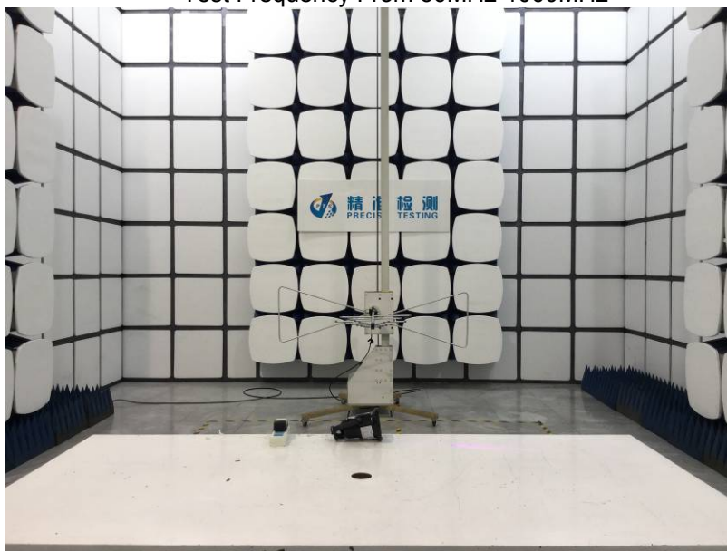
Radiated Spurious Emissions Test Frequency From 30MHz-1000MHz
