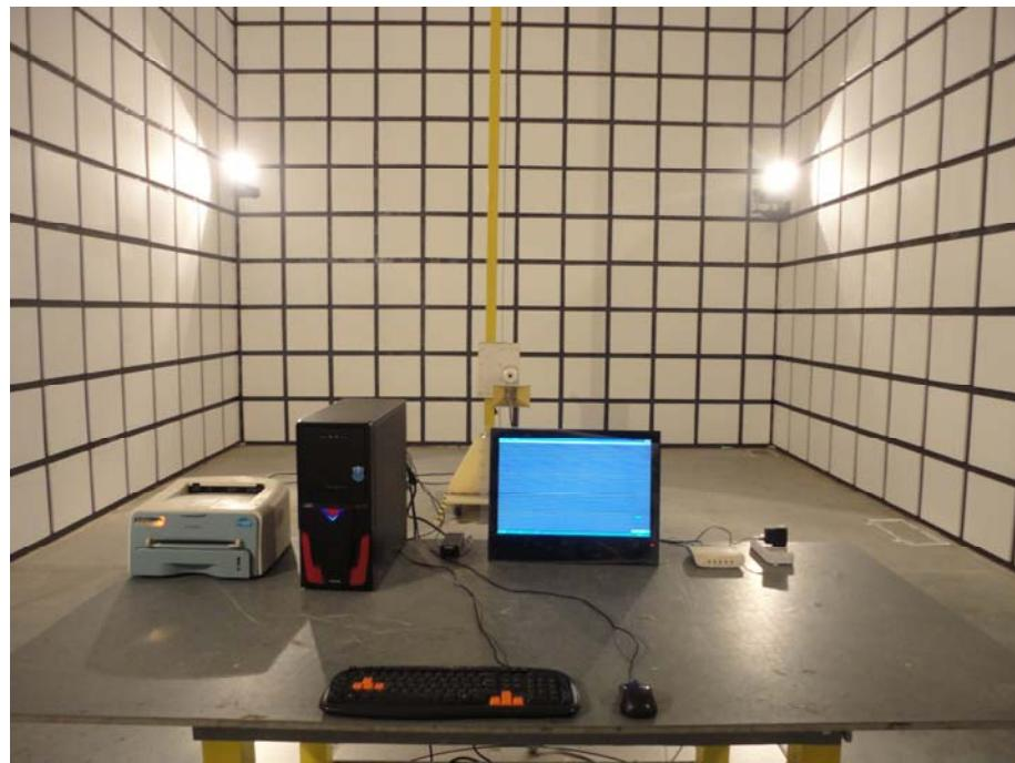
**RADIATED EMISSION TEST (PC BY VGA)**
