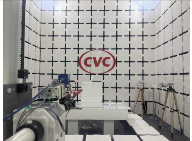
PRO25T-6S-IOT RE (Above 1GHz-outdoor)
