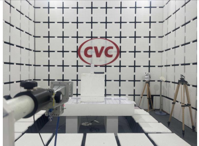
PRO25T-6S-IOT RE (Above 1GHz-outdoor)
