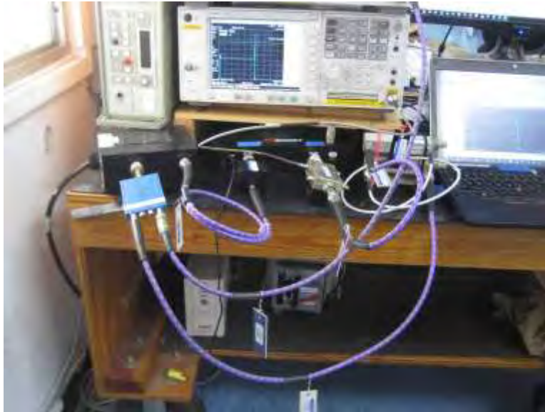
Section 7.11 Oscillation Mitigation (Notch Filter) Test Setup
