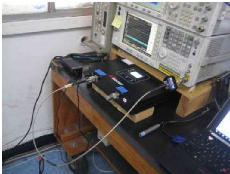
Section 7.7 Max Noise Uplink Test Setup
