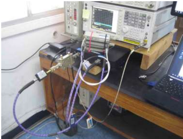
Section 7.11 Oscillation Timing Test Setup
