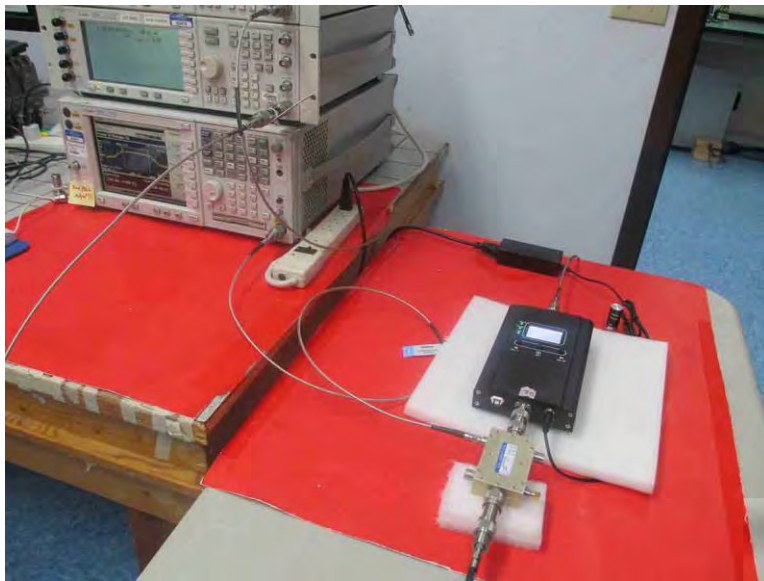
Section 7.9.2 Variable Gain Test Setup
