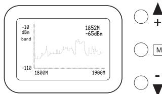
As shown in the figure above, the testing frequency band range is 1800~1900MHz, and testing signal power range is -10dBm~ -110dBm, the signal reference point is 1852M, the power of the reference point is -65dBm.
