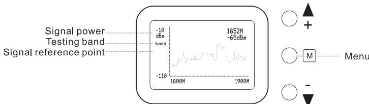
**Band:** Displays the testing frequency bands where the amplifier is operating (adjustment accuracy:100MHz/1step).
