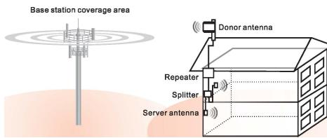
Figure 1: Application diagram
