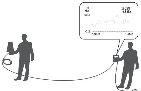
The outdoor antenna receives the strongest signal when the signal power reaches relatively highest level. If the LCD shows a maximum power at present, it means the present location is the best for ensuring that the booster has maximized performance.
