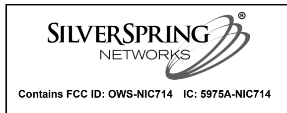
Figure 9. Sample FCC ID label for devices containing a NIC
