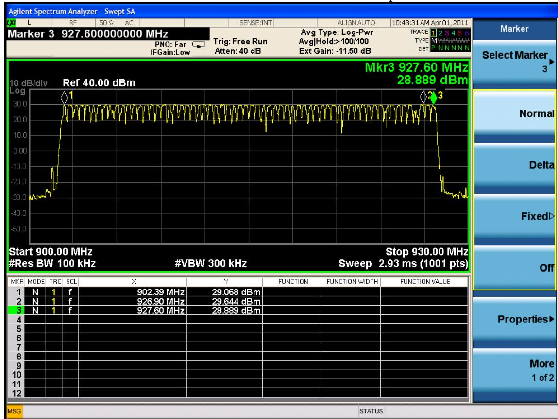
**NUMBER OF HOPPING CHANNELS: 300 kHz Channel Separation**
