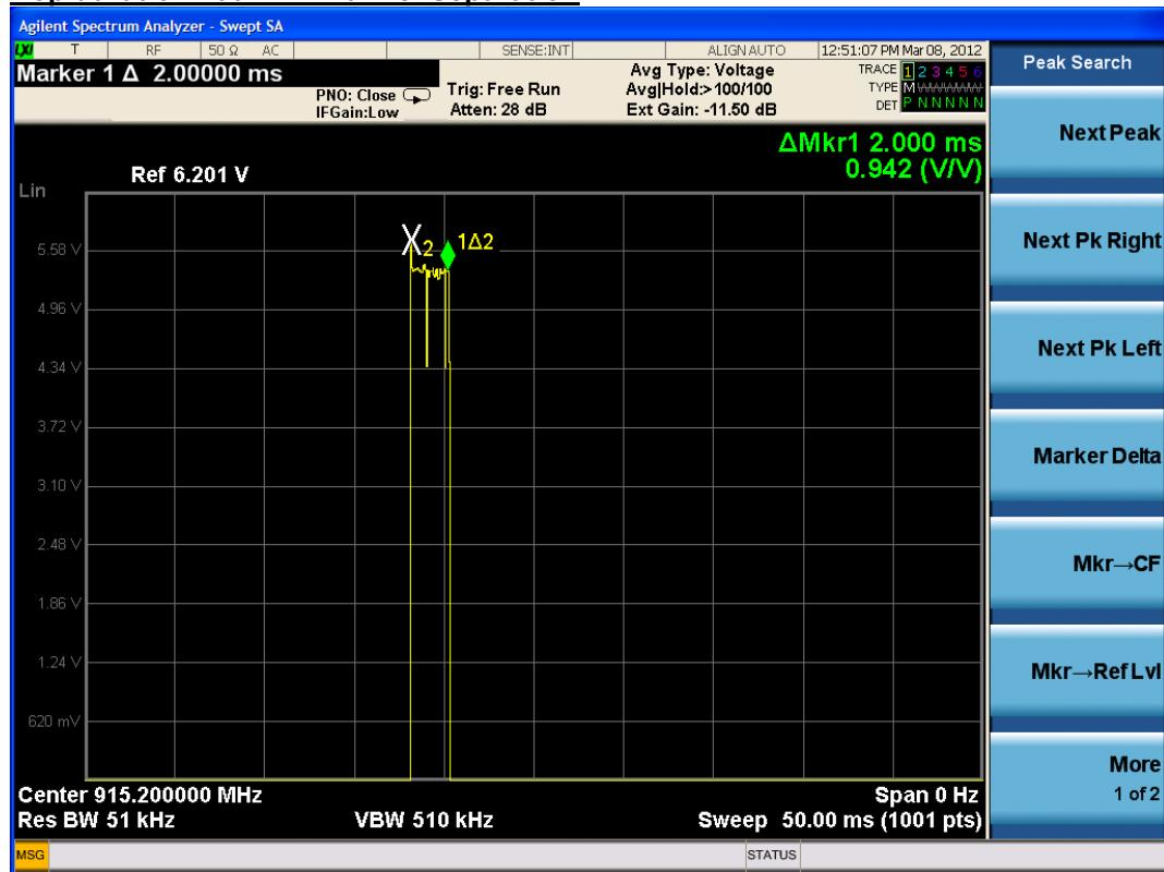
**NUMBER OF PULSES IN 20 SECOND OBSERVATION PERIOD 200kHz Channel Separation**
