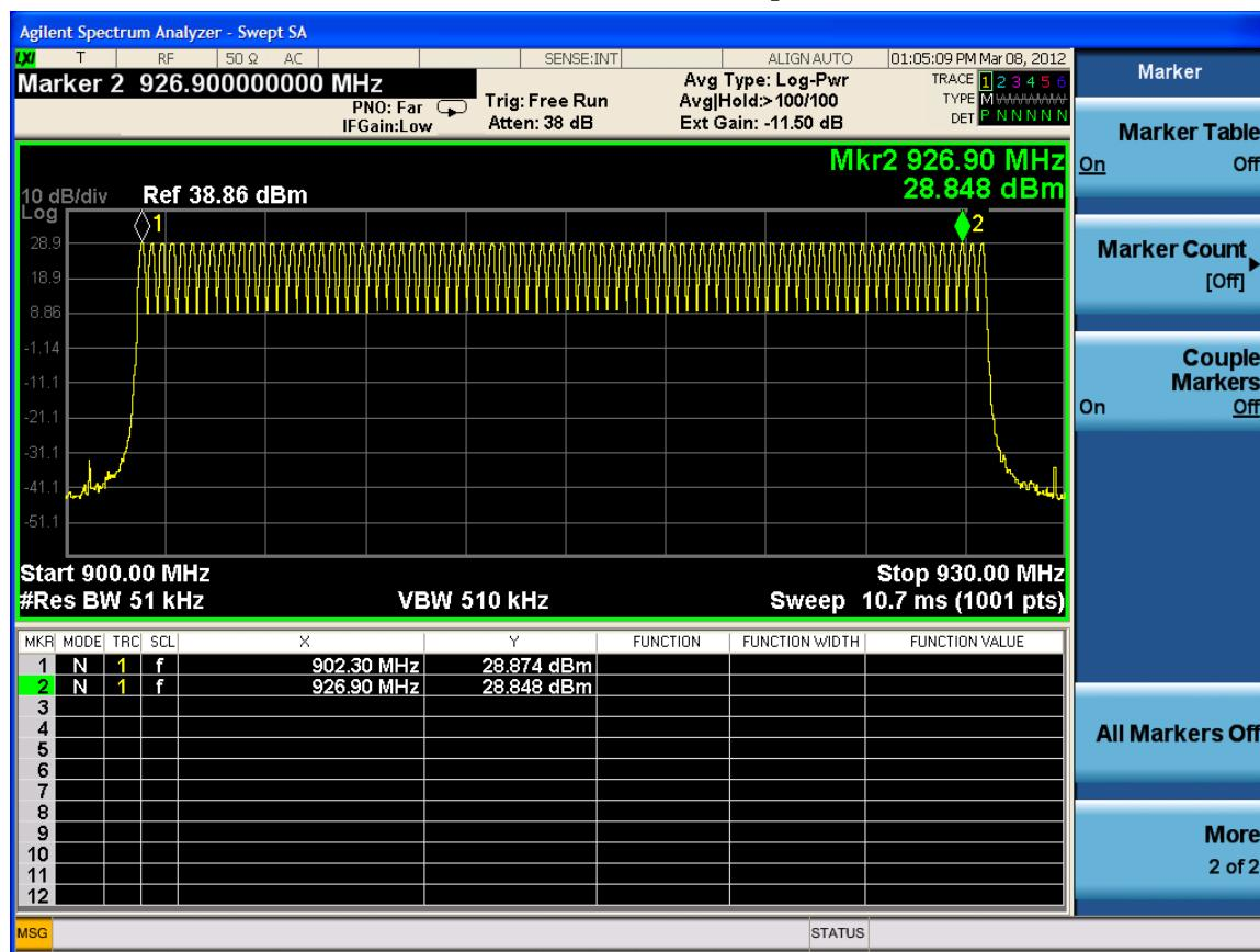
**NUMBER OF HOPPING CHANNELS: 200 kHz Channel Separation**
