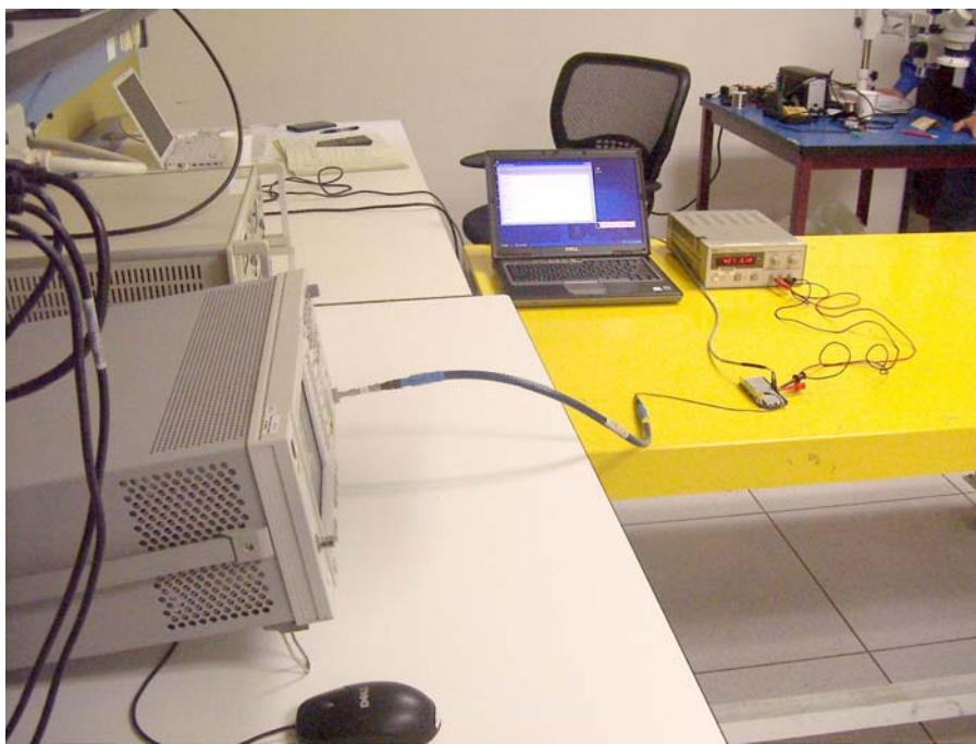
**RADIATED RF MEASUREMENT SETUP**
