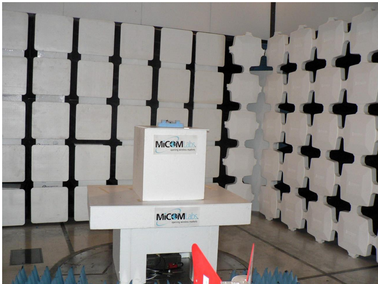
ITRO01 NIC-510 with Integral Antenna Tx Spurious Front 1-18G
