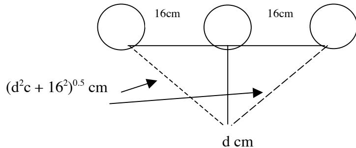
At a point located a distance  $d$  from a meter module antenna, the power density is the sum of the contributions from the center meter and the two adjacent meters. Each adjacent meters is further away, at a distance of  $(d^2c + 16^2)^{0.5}$  cm, and therefore will contribute less power density at  $d$  for the same transmitter eirp.
