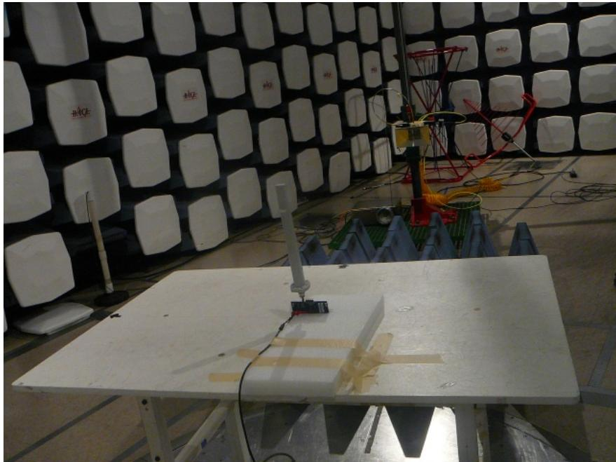
Radiated emissions – L-Com Antenna
