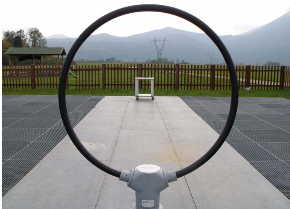
Figure 3: Radiated emission test – under 30 MHz on OATS
