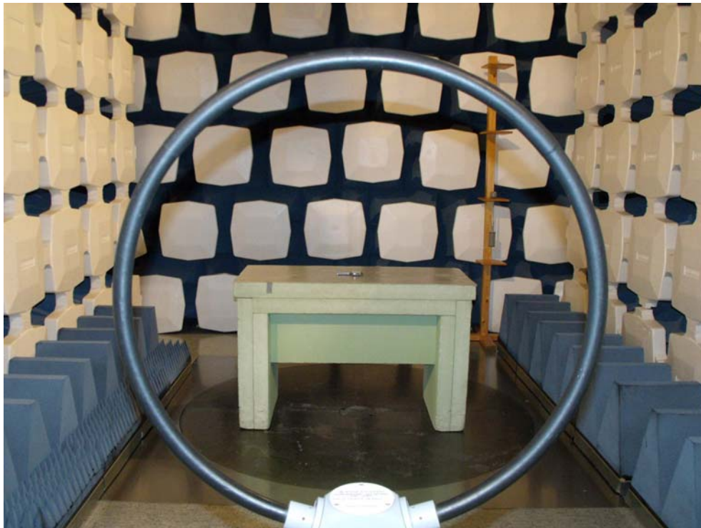
Figure 1: Radiated emission test – under 30 MHz
