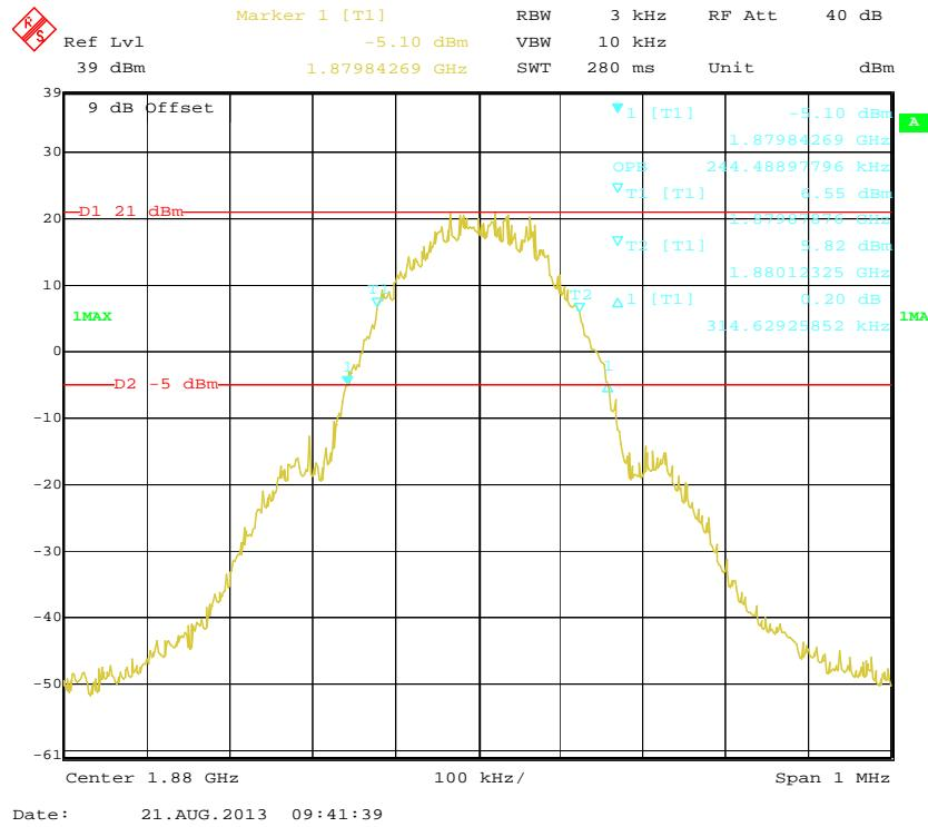
**FCC §2.1051, §22.917(a) & §24.238(a) - SPURIOUS EMISSIONS AT ANTENNA TERMINALS****Applicable Standard**
