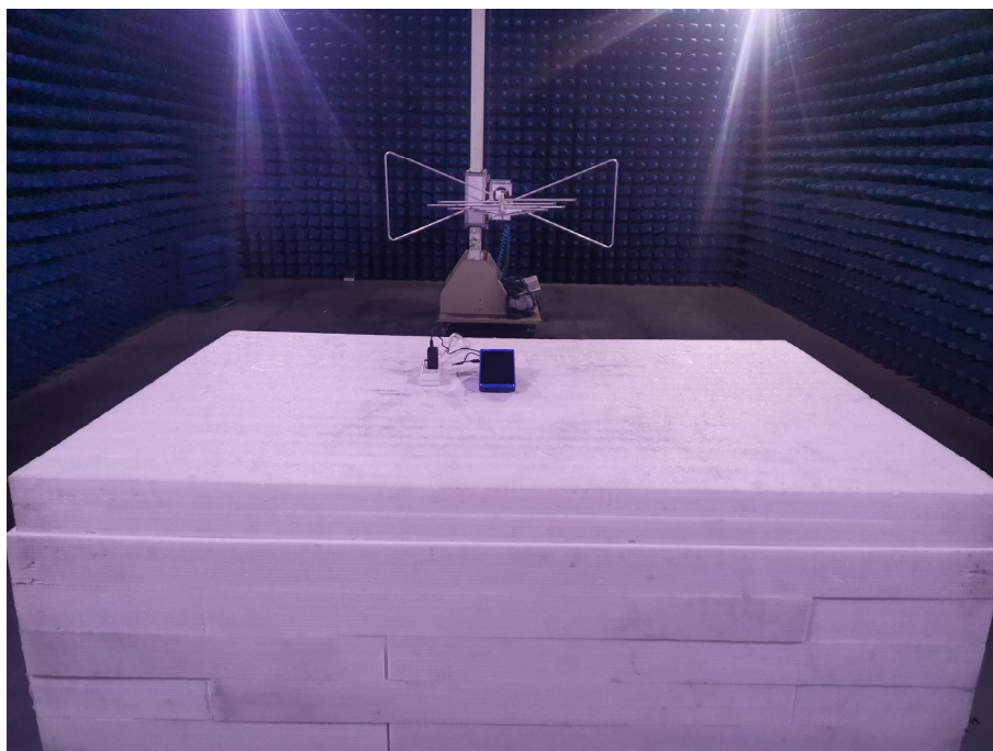
Photo of Radiated Emission Measurement (Below 1G)
