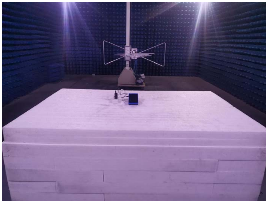
Photo of Radiated Emission Measurement (Below 1G)
