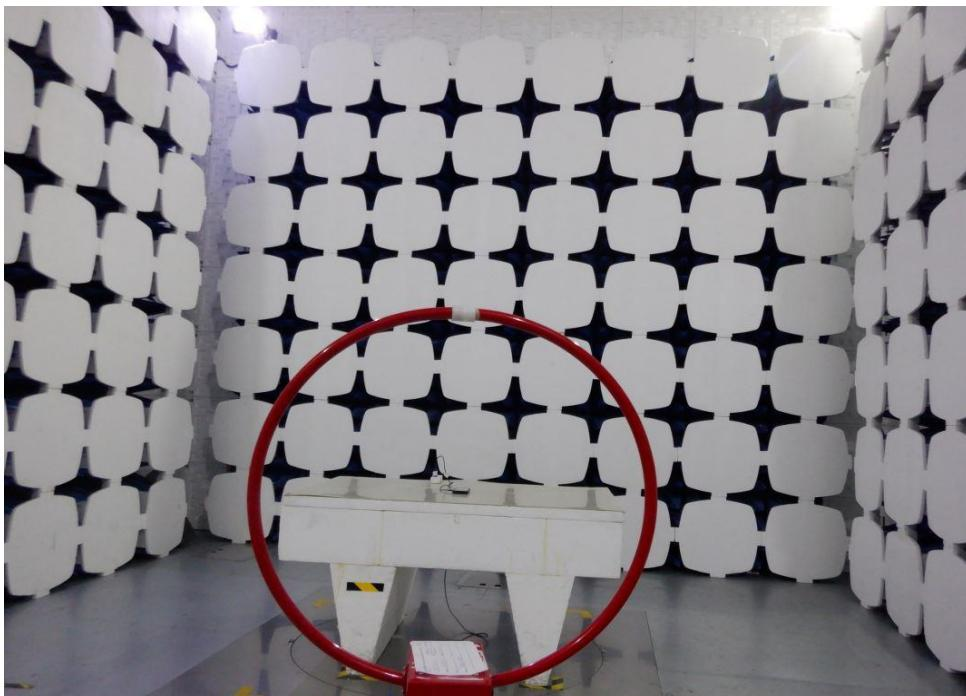
**Radiated Spurious Emissions Below 1GHz (30MHz-1GHz)**
