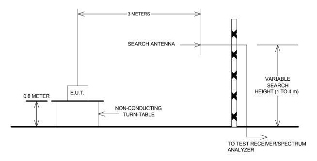
The spectrum was searched up to the 10th harmonic of the fundamental frequency of operation.
