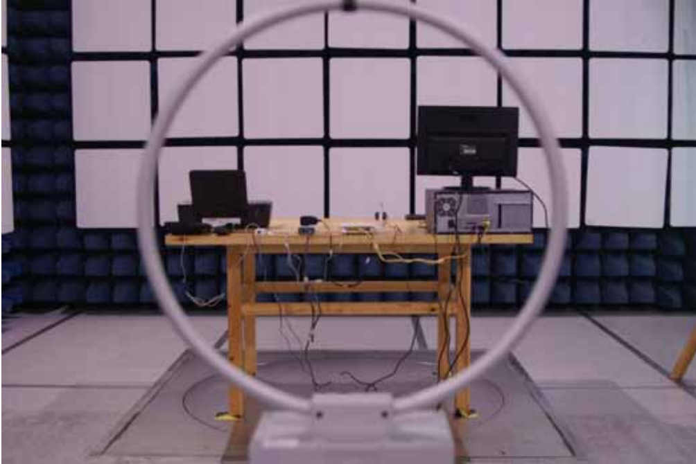
Below 30MHz (The Adapter DSA-12CA-12 120100)
