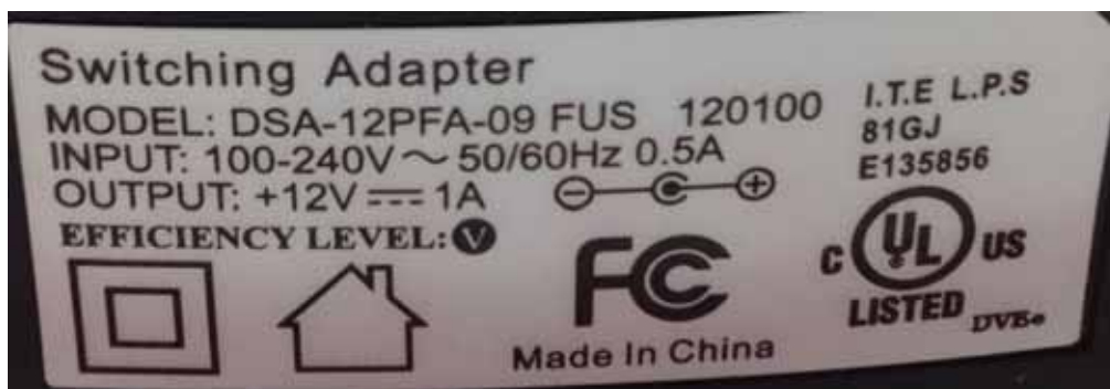
THE LABEL OF ADAPTER DSA-12PFA-09 FUS 120100
