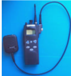
speaker/microphone with antenna port, black, Ericsson, CSA/FM KRY 101 1617/84 (left)
