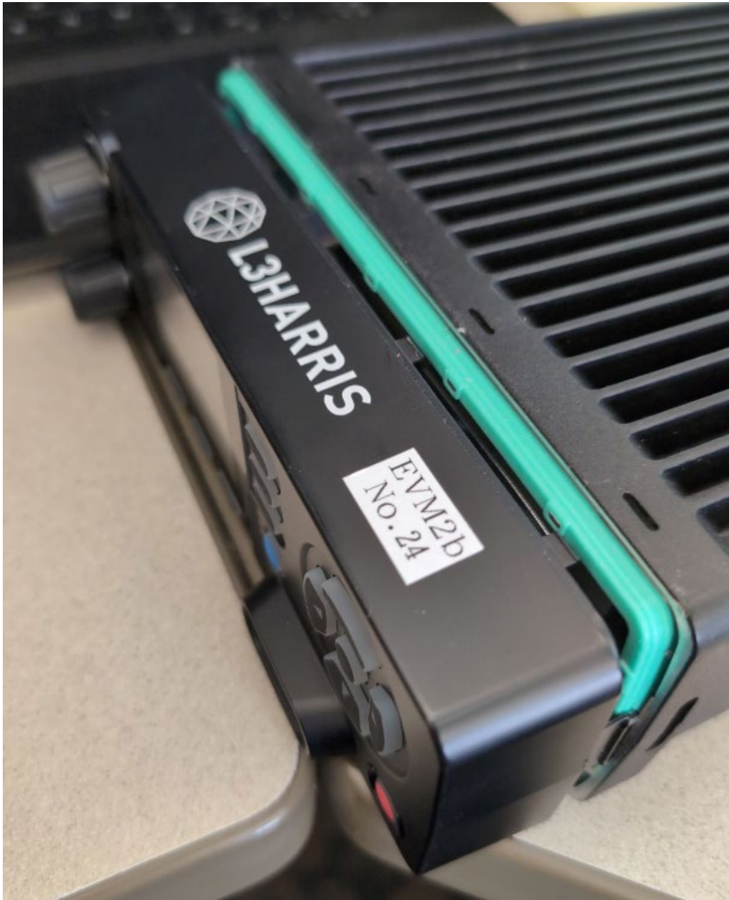
Photo 9: XL-CH2 Control Head (left) partially separated from XL-85M
