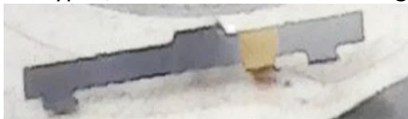
Photo 11: BT/WiFi Antenna, front and back views. Gold area indicates contact point with the spring-loaded pin on Keypad/LCD Solder Side connecting BT/WiFi antenna to PWB BT/WiFi trace (see Photo 9)
