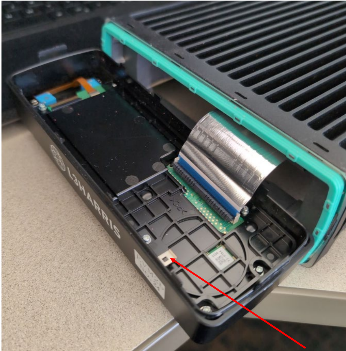
Visible portion of BT/WiFi antenna when Keypad/LCD board inside Keypad front cover
