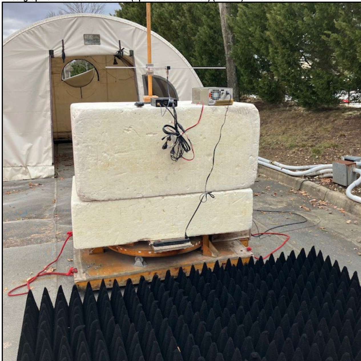
Photograph 3: Radiated Emissions (Spurious/Harmonics) (>1 GHz) – Front View
