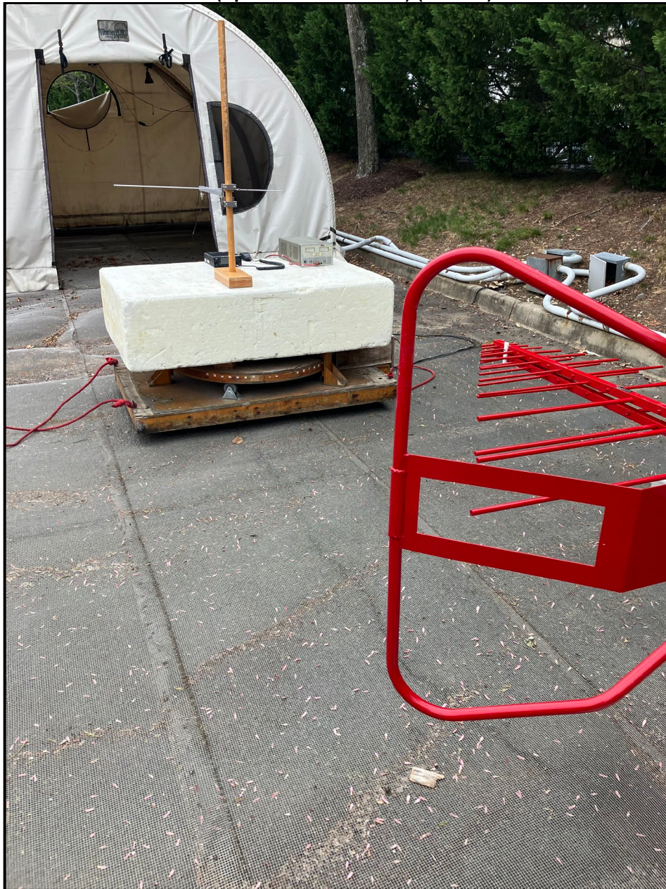
Photograph 1: Radiated Emissions (Spurious/Harmonics) (<1 GHz) - Front View
