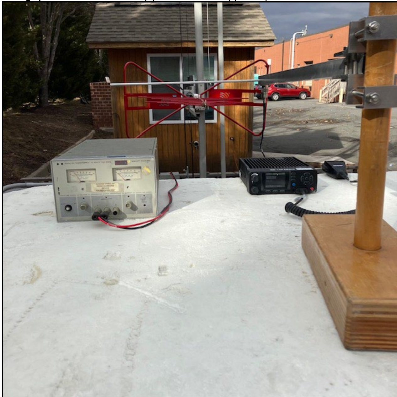
Photograph 4: Radiated Emissions (Spurious/Harmonics) (>1 GHz) – Back View
