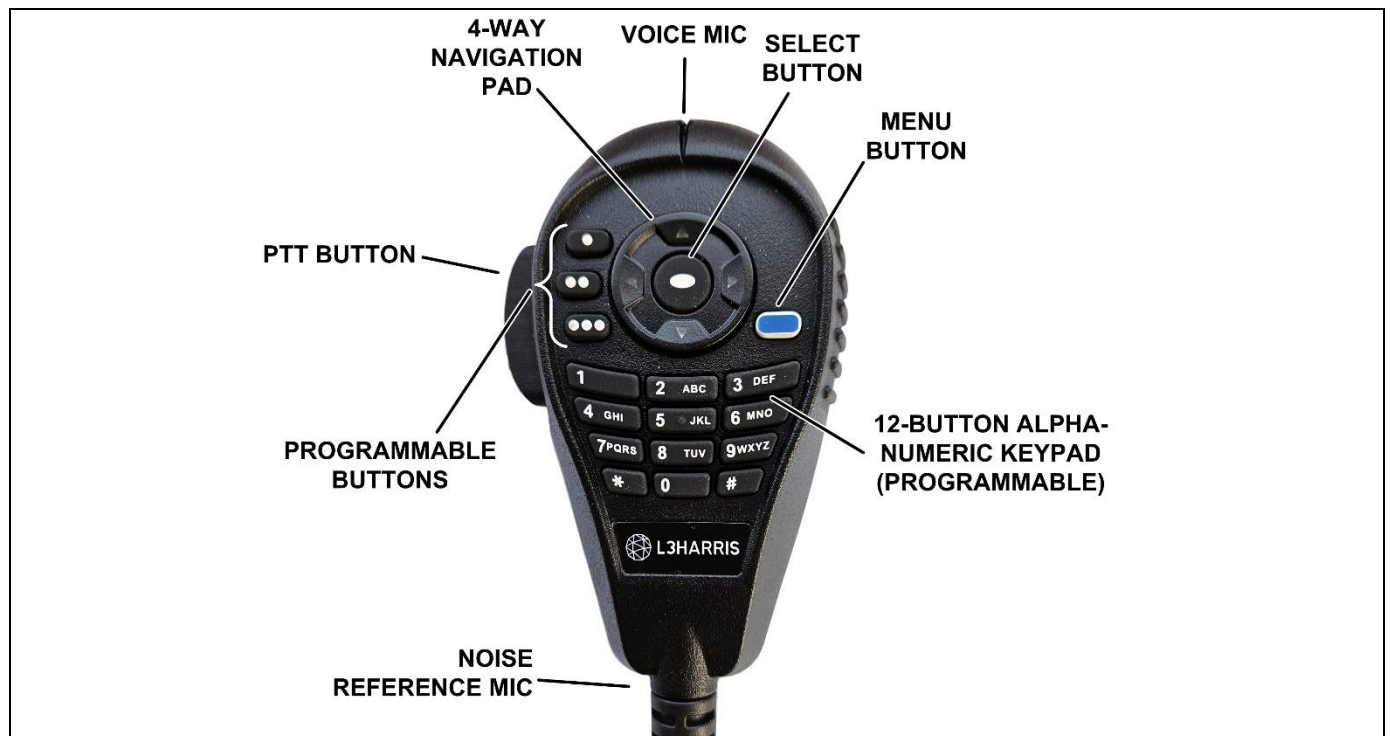
Figure 4-2: Keypad Mobile Microphone (KMM) Controls
