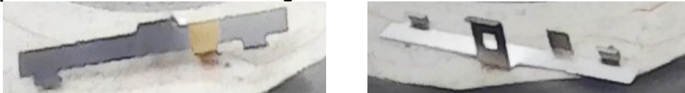
BT/WiFi Antenna, front and back views. Gold area indicates contact point with the spring-loaded pin on Keypad/LCD Solder Side connecting BT/WiFi antenna to PWB BT/WiFi trace
