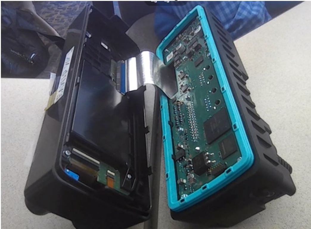
XL-CH2 Opened – Internal View; Keypad/LCD Board on left under plastic cover with attached BT/WiFi antenna; Main Board Solder Side visible on right
