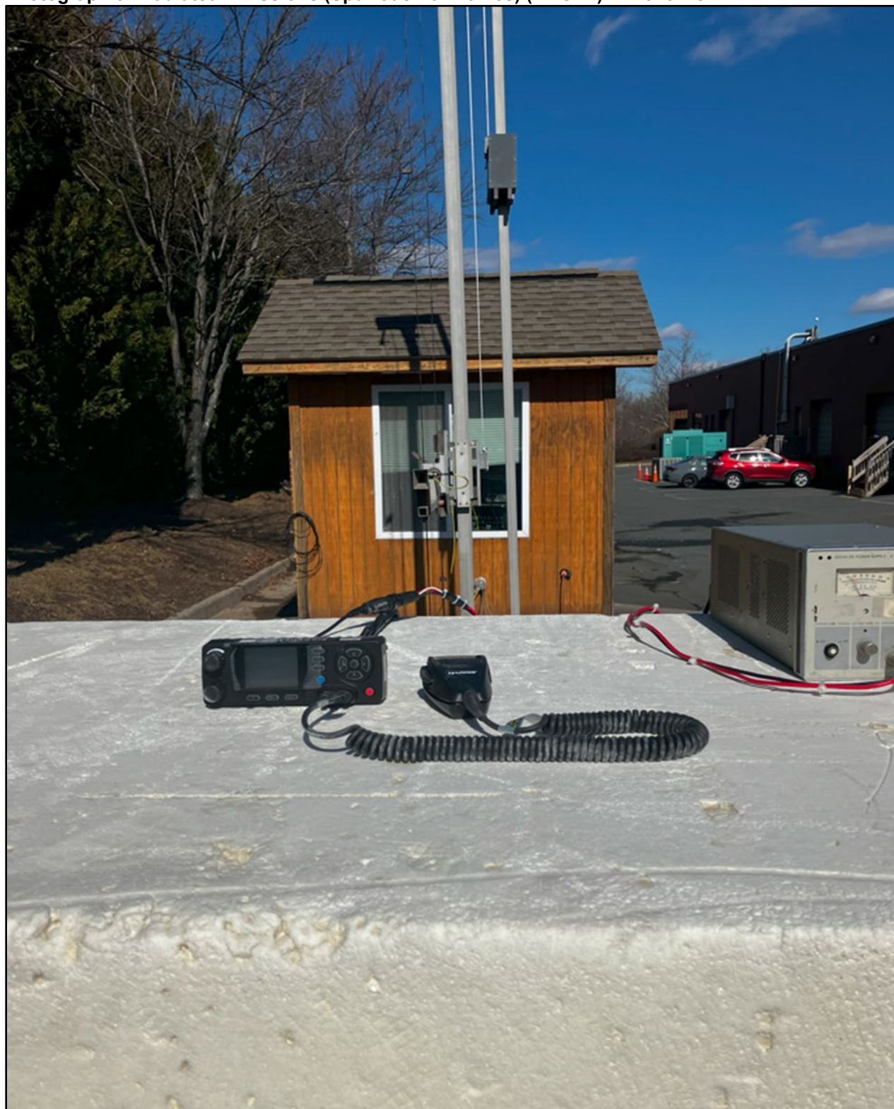
Photograph 3: Radiated Emissions (Spurious/Harmonics) (>1 GHz) – Front View
