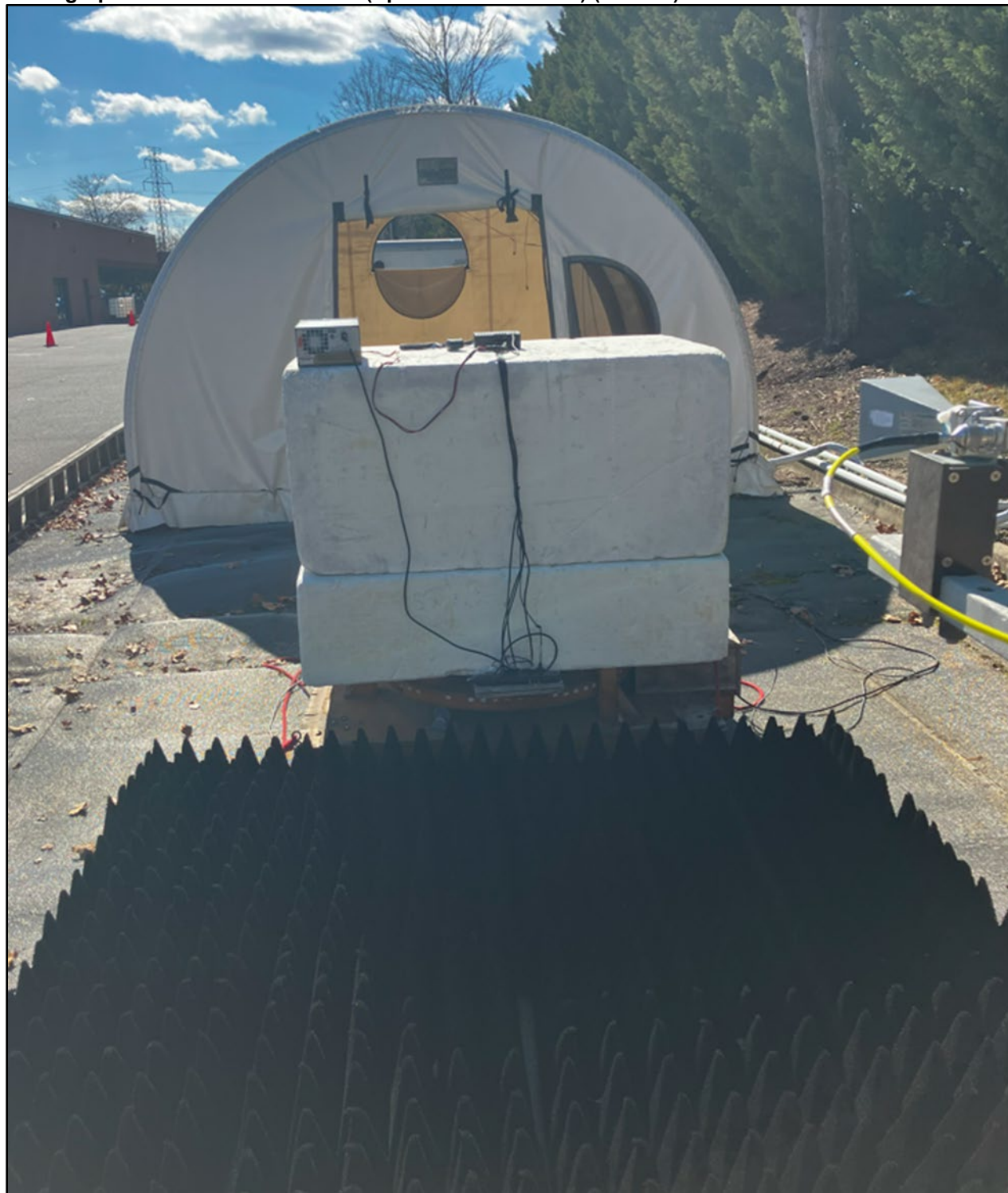
Photograph 4: Radiated Emissions (Spurious/Harmonics) (>1 GHz) – Back View
