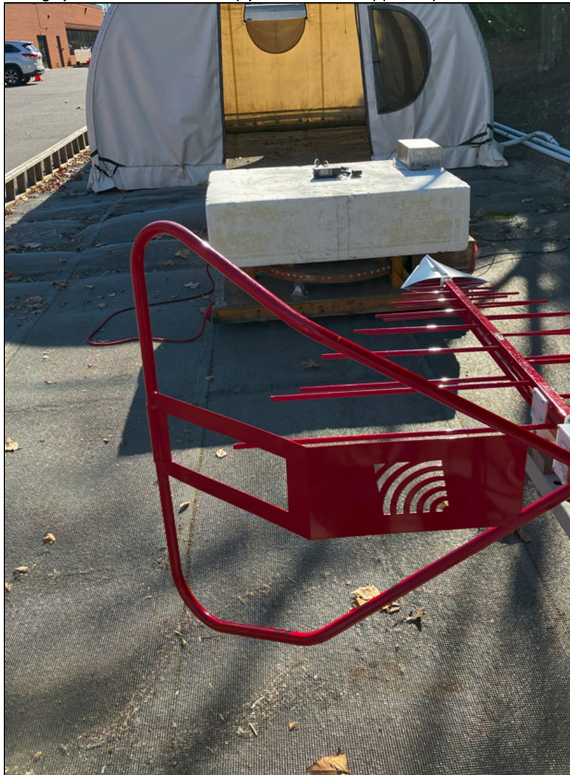
Photograph 1: Radiated Emissions (Spurious/Harmonics) (<1 GHz) - Front View
