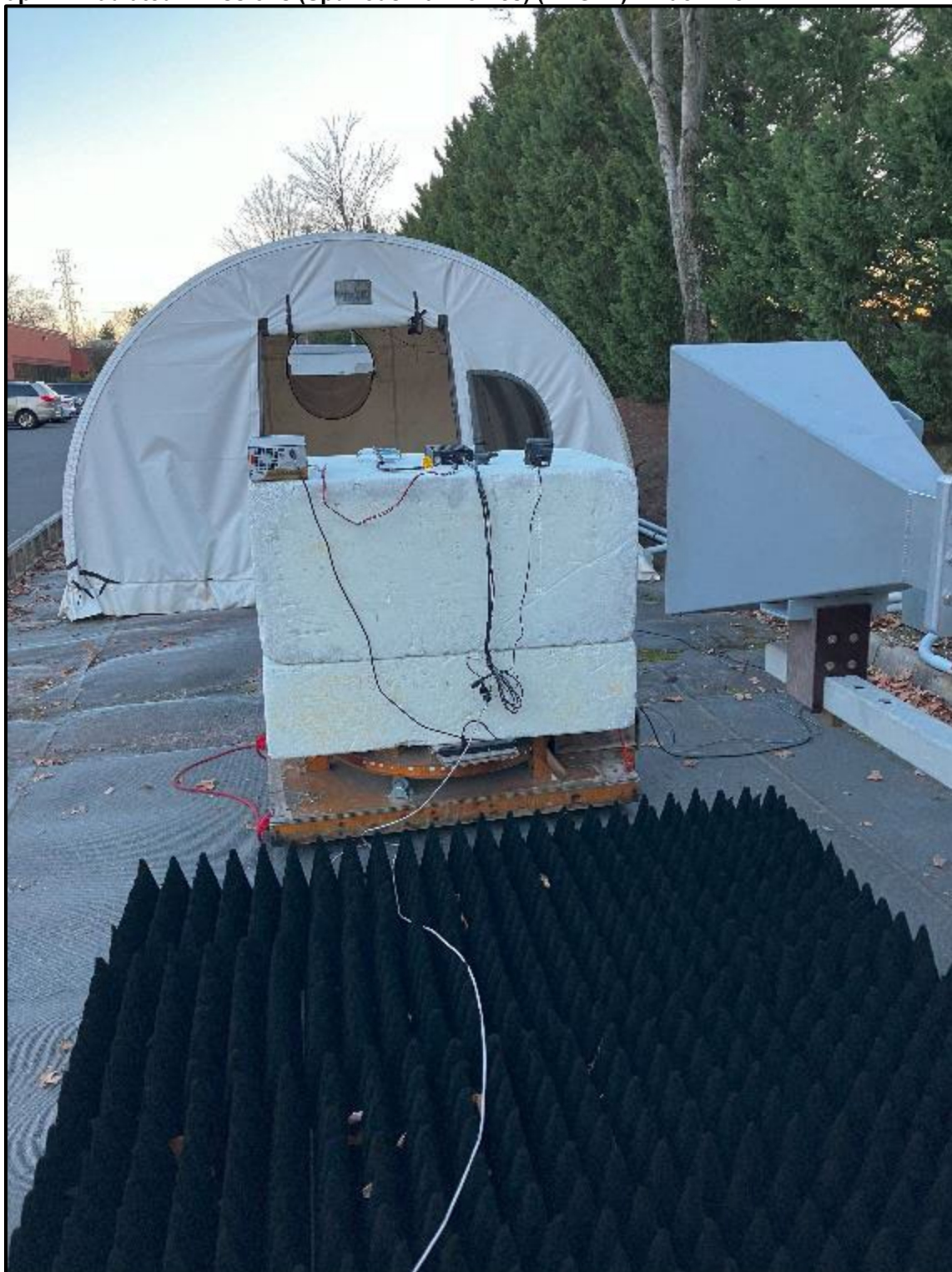
Photograph 4: Radiated Emissions (Spurious/Harmonics) (>1 GHz) – Back View
