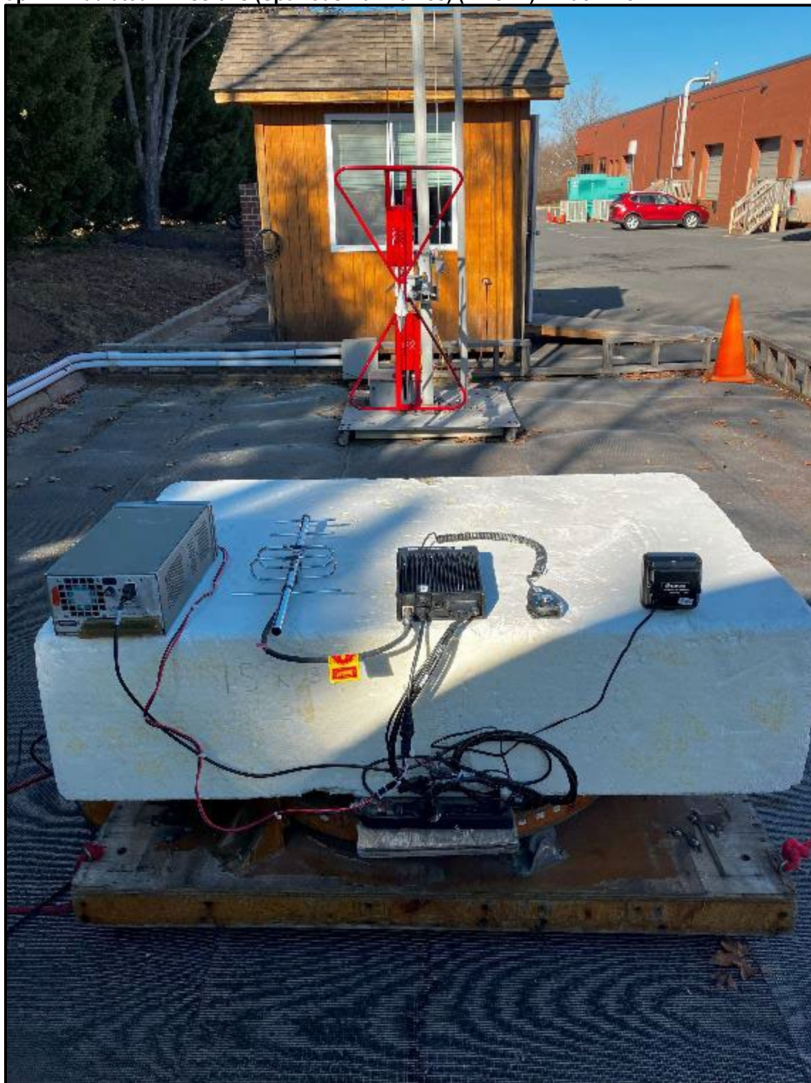
Photograph 2: Radiated Emissions (Spurious/Harmonics) (<1 GHz) – Back View
