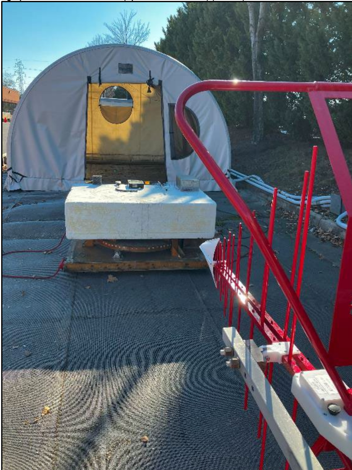
Photograph 1: Radiated Emissions (Spurious/Harmonics) (<1 GHz) - Front View
