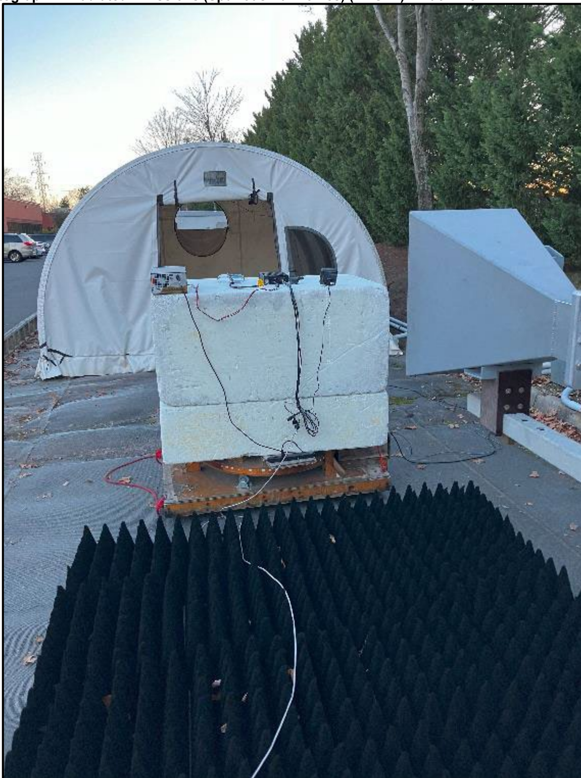
Photograph 4: Radiated Emissions (Spurious/Harmonics) (>1 GHz) – Back View
