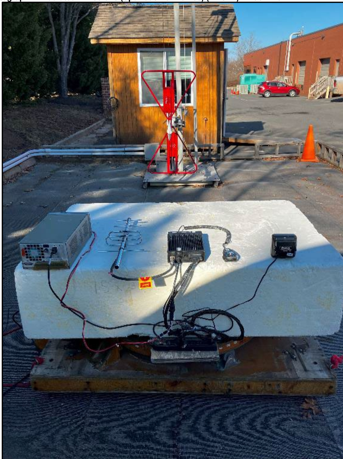
Photograph 2: Radiated Emissions (Spurious/Harmonics) (<1 GHz) – Back View
