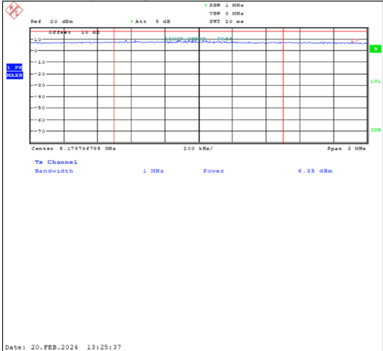
Plot 7-1: Power Spectral Density – 5180 MHz – 802.11a
