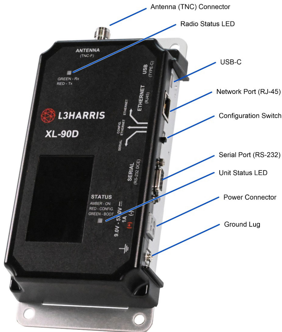
Figure 4-1: XL-90D Indicators and Controls
