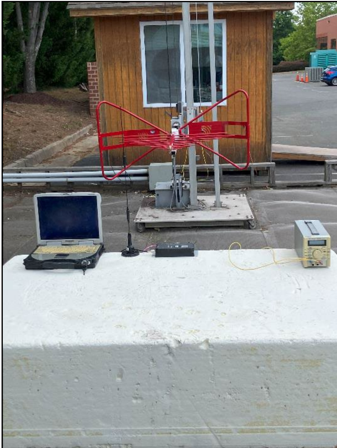
Photograph 3: Radiated Emissions (Spurious/Harmonics) Under 1 GHz, Front View
