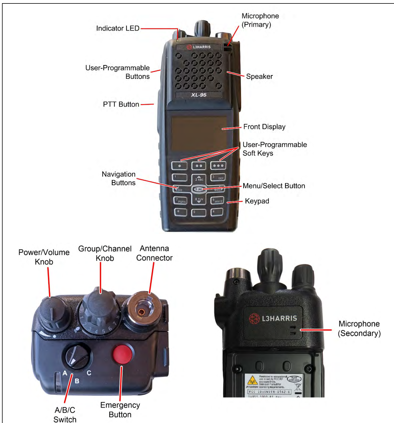
Figure 4-1: Radio Controls, Indicators, and Connectors
