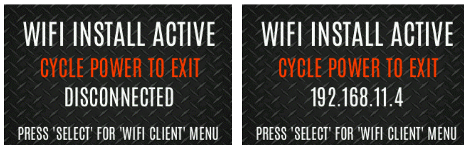
Figure A-5: Enable Wi-Fi Programming Mode on Radio
