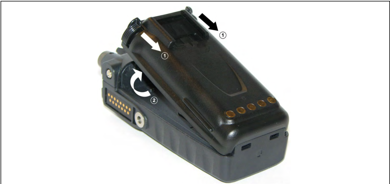
Figure 3-2: Remove the Battery
