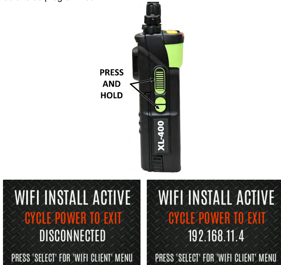
Figure 12-5: Enable Wi-Fi Programming Mode on Radio
