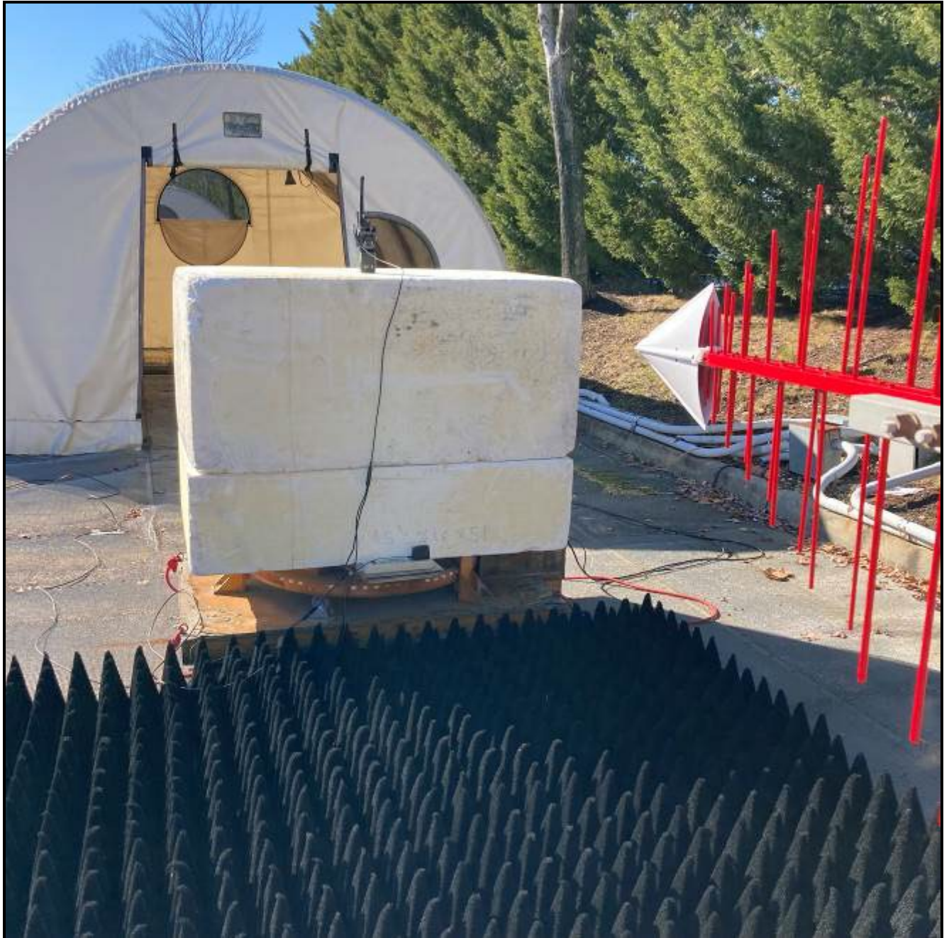
Photograph 2: Radiated Emissions (Spurious/Harmonics) Over 1 GHz, Back View
