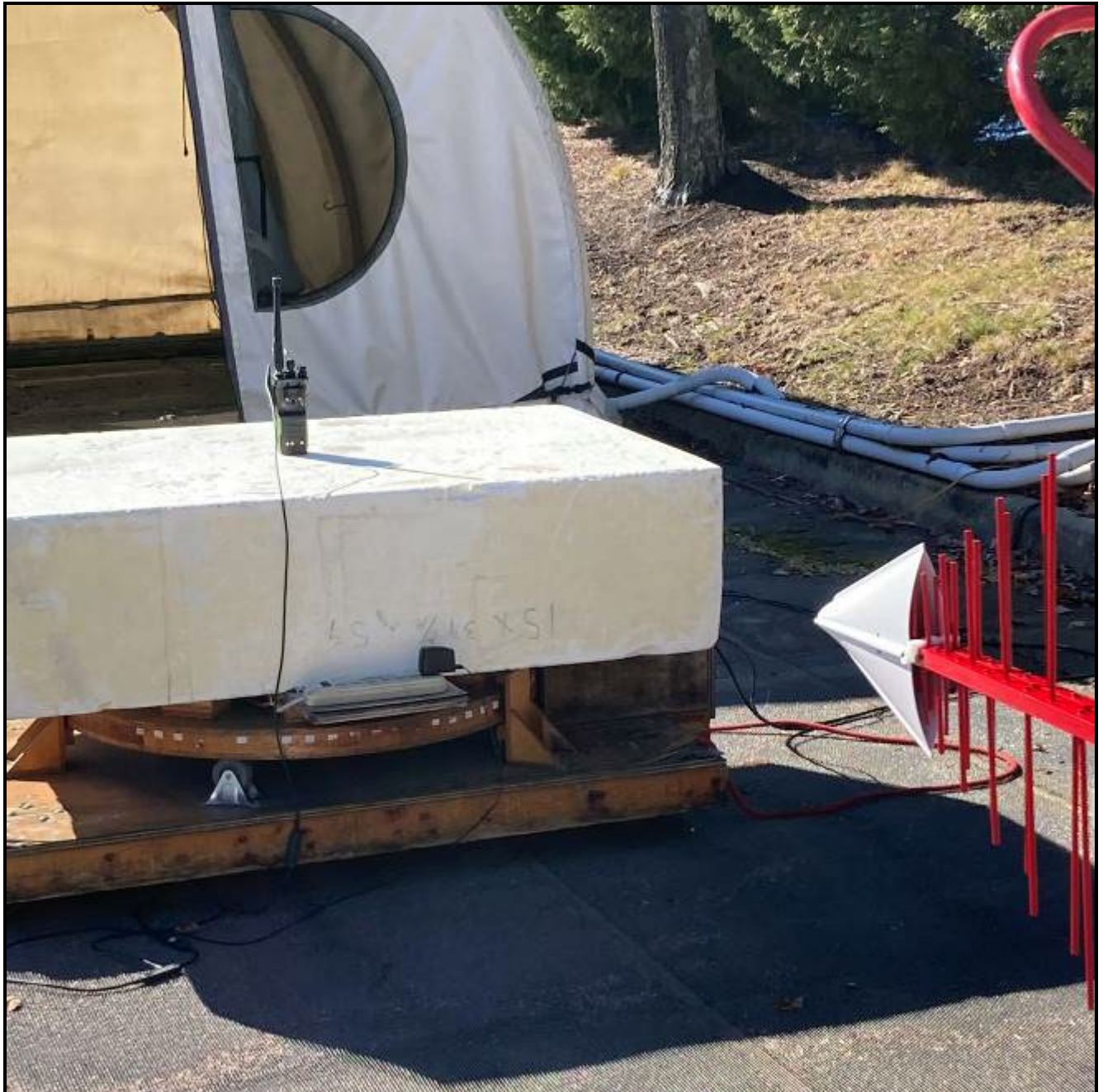
Photograph 4: Radiated Emissions (Spurious/Harmonics) Under 1 GHz, Back View
