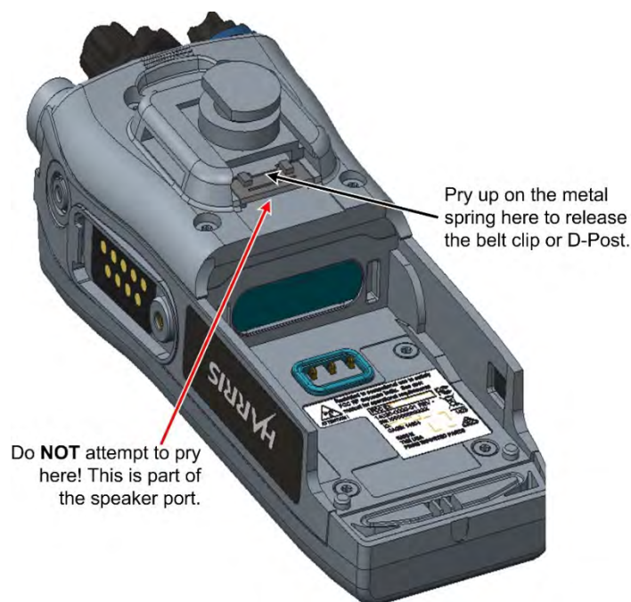
Figure 4-3: Remove Belt Clip
