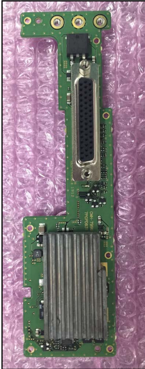
Connector Board Back View with Heatsink
