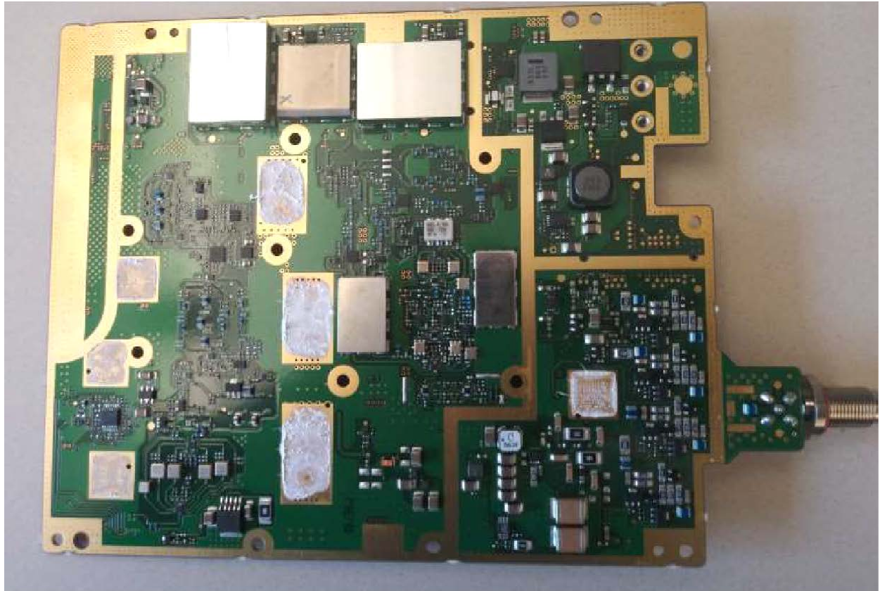
VCH RF Board Solder Side with Shields
