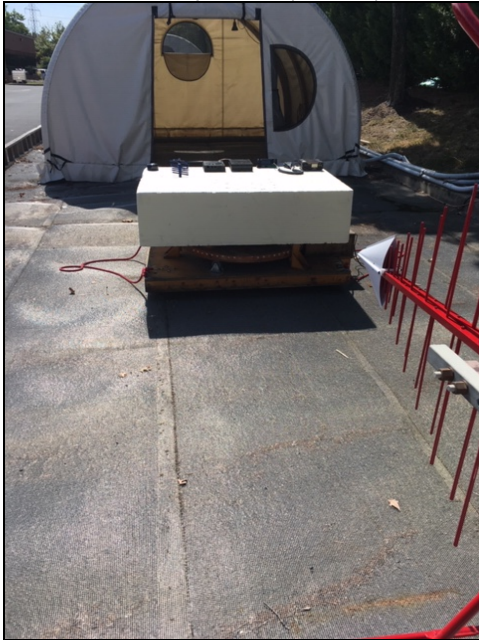
Photograph 3: Radiated Emissions Testing – Front View (Below 1 GHz)
