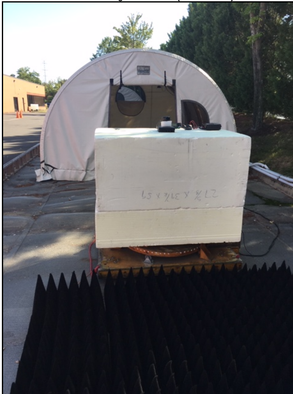
Photograph 1: Radiated Emissions Testing – Front View (Above 1 GHz)
