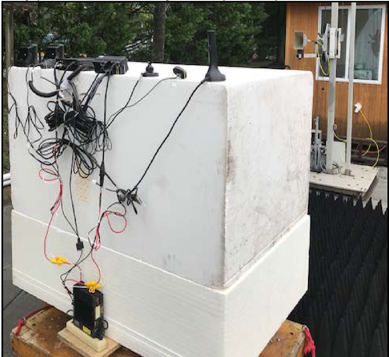
Photograph 2: Radiated Emissions Testing – Back View (Above 1 GHz)
