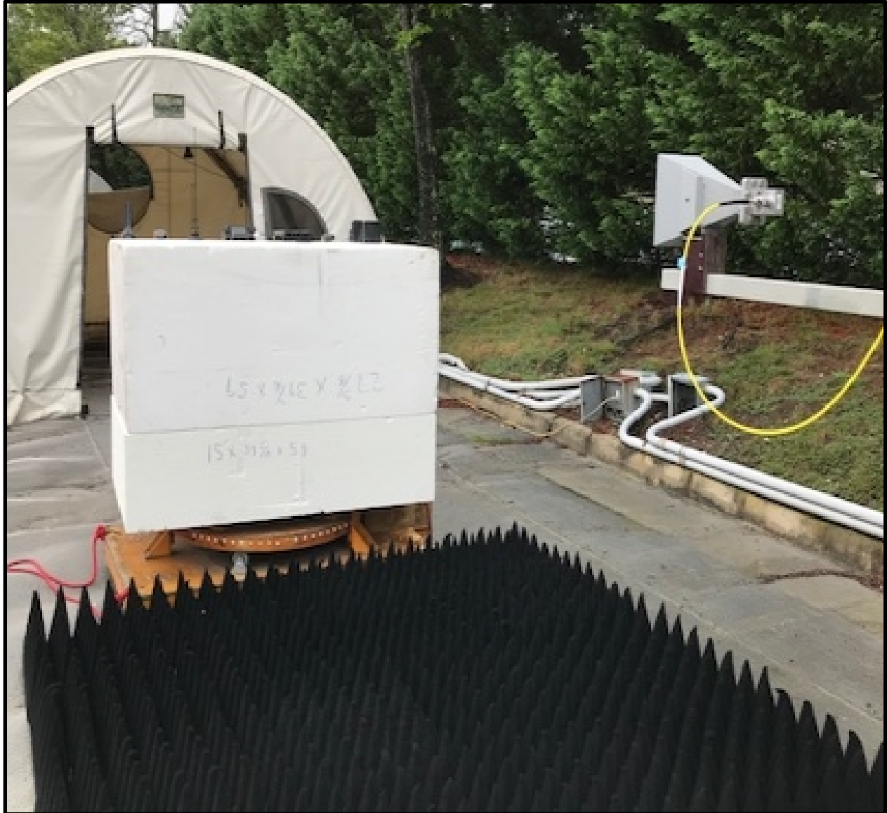
Photograph 1: Radiated Emissions Testing – Front View (Above 1 GHz)
