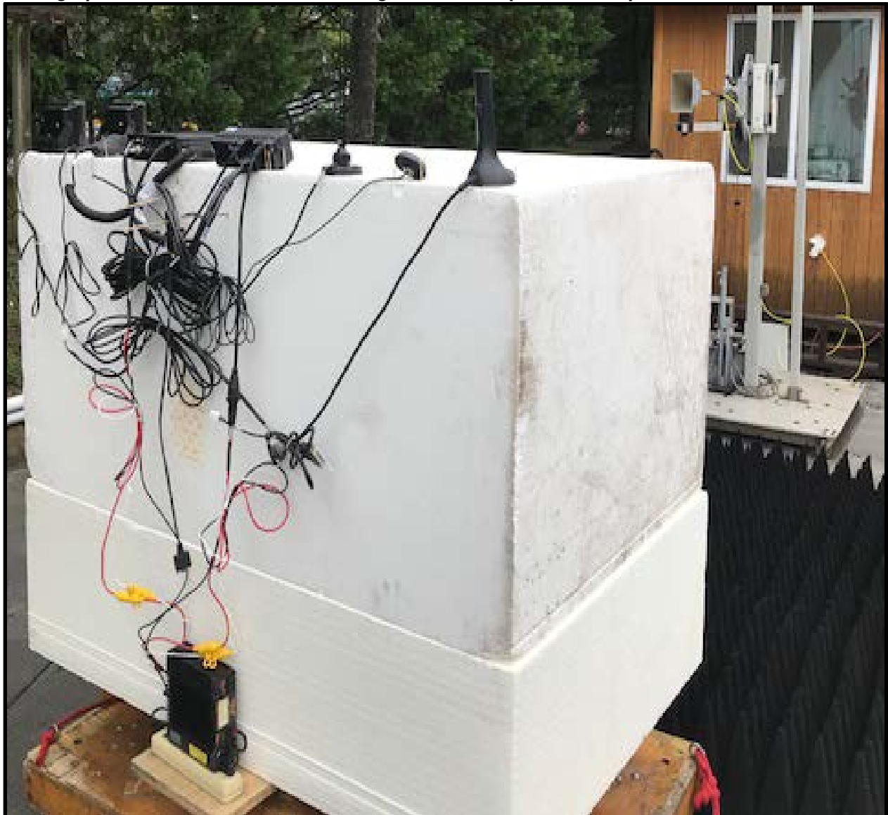
Photograph 2: Radiated Emissions Testing – Back View (Above 1 GHz)
