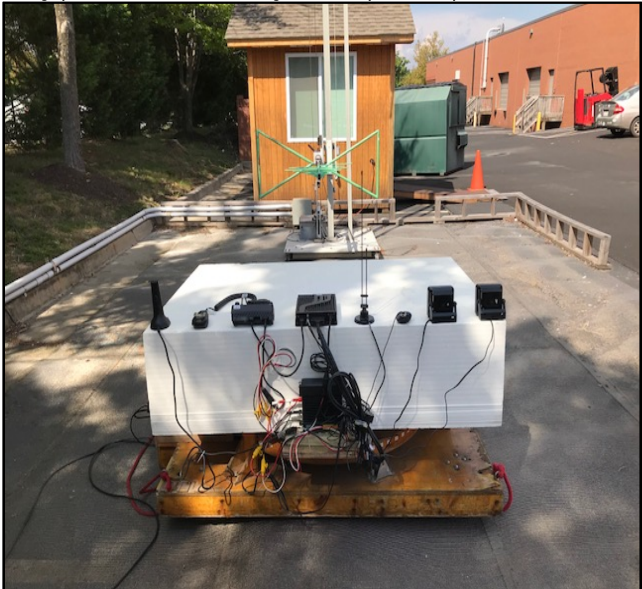
Photograph 4: Radiated Emissions Testing – Back View (Below 1 GHz)
