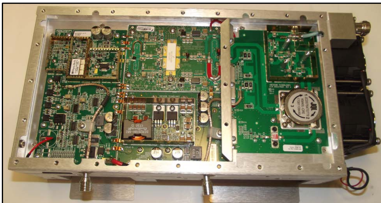
Power Amplifier Top View No Shields
