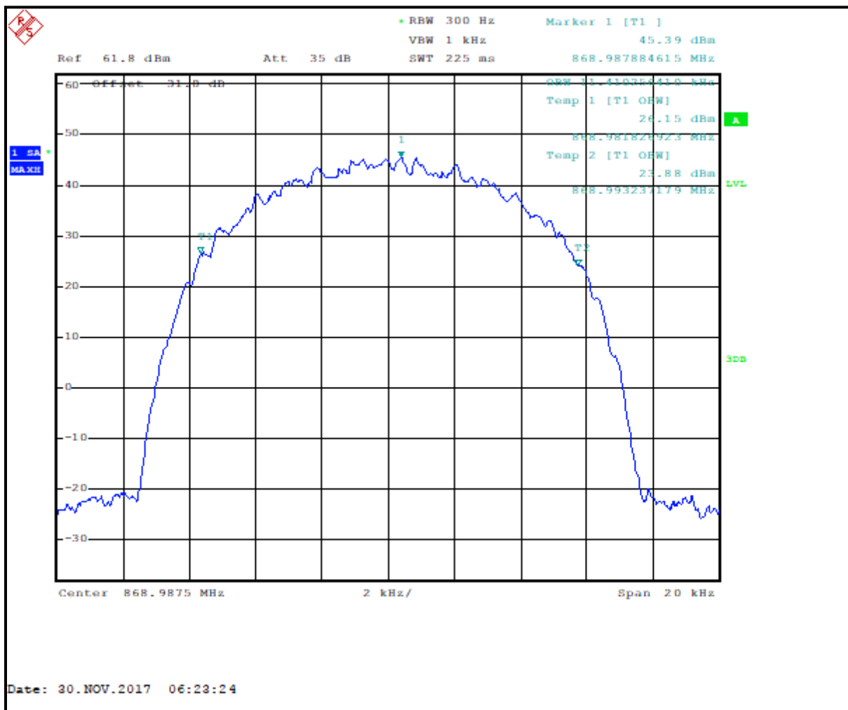
Plot 7-48: Occupied Bandwidth – 868.9875 MHz; HDQPSK; 20 dB BW
