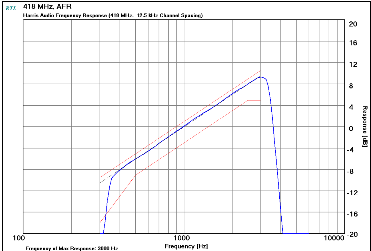
Plot 9-1: Modulation Characteristics - Audio Frequency Response - 418 MHz
