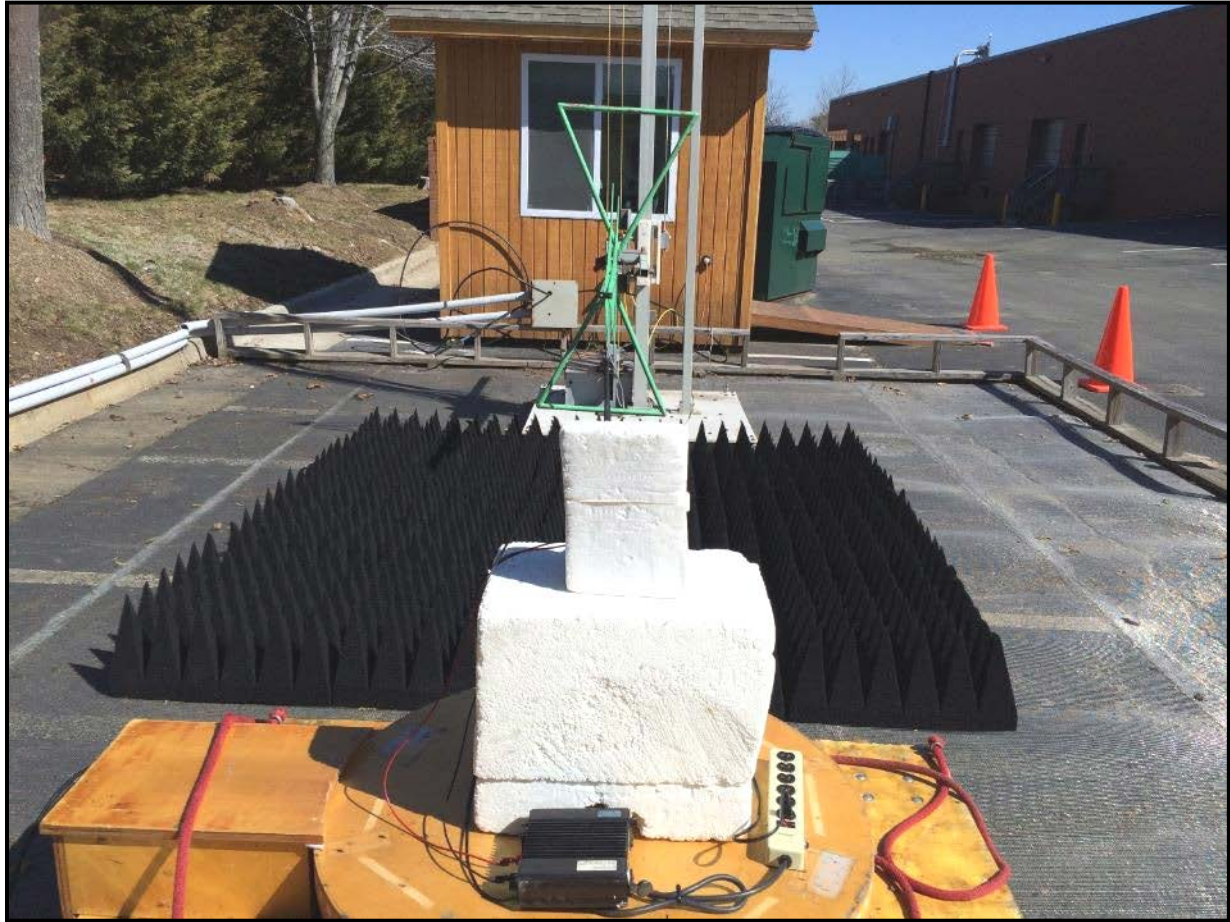
Photograph 2: Radiated Emissions Testing – Back View
