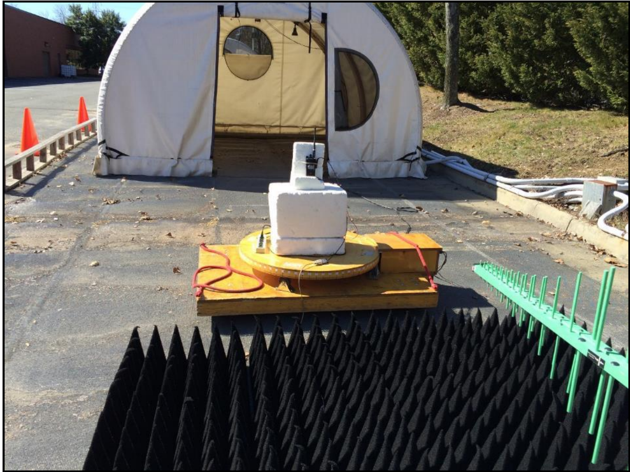
Photograph 1: Radiated Emissions Testing – Front View
