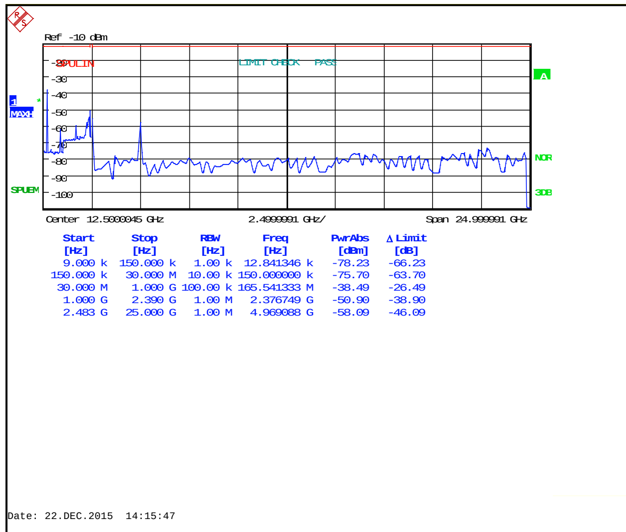
Plot 5-3: Antenna Conducted Spurious Emissions – 2480 MHz
