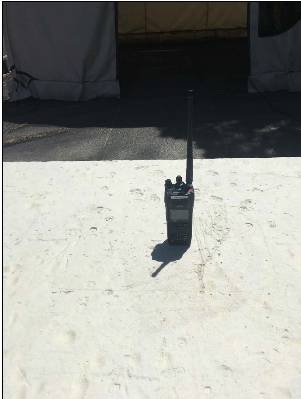
Photograph 3: Radiated Emissions (Spurious/Harmonics) Under 1 GHz, Front View
