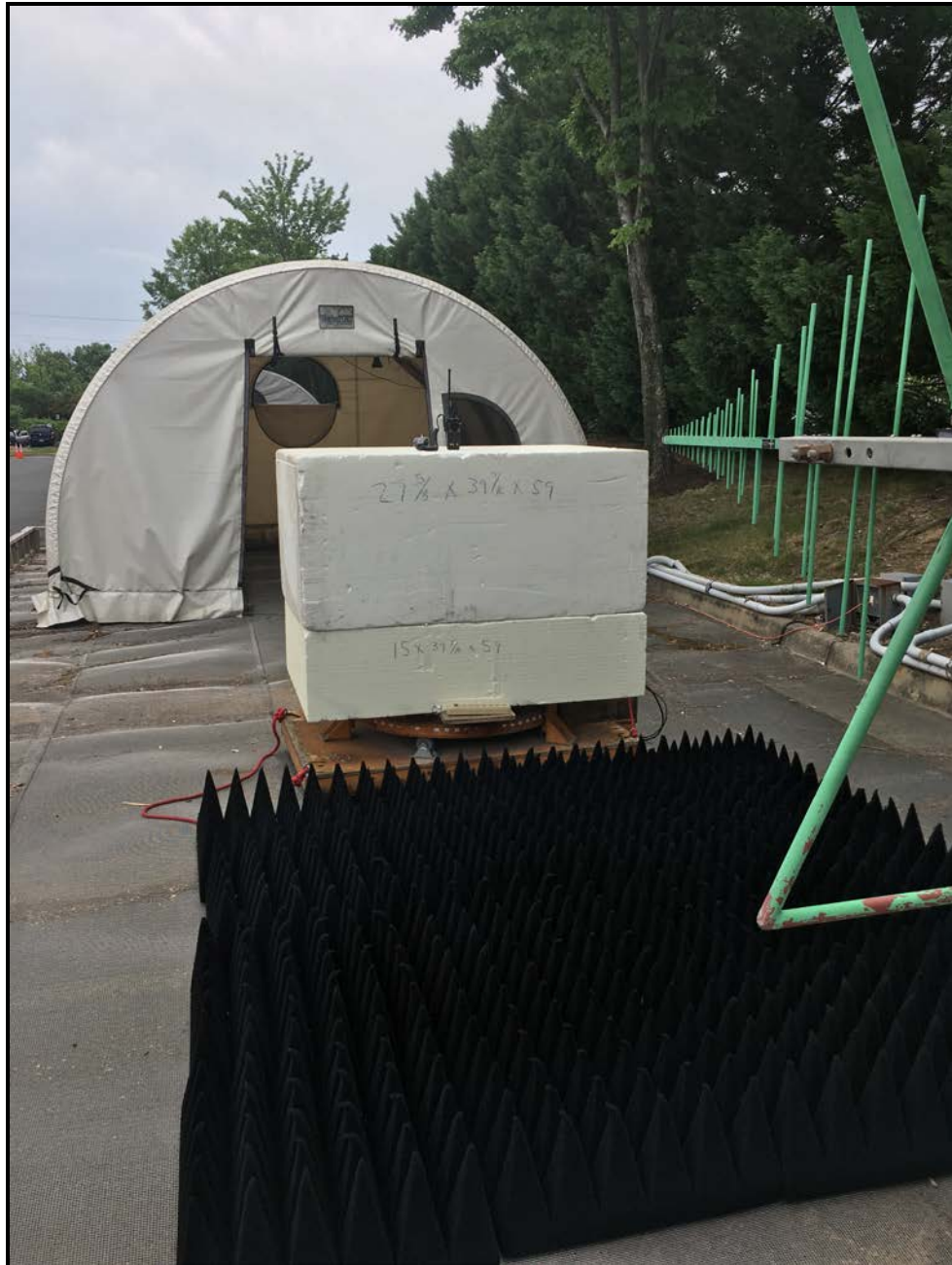
Photograph 2: Radiated Emissions (Spurious/Harmonics) Over 1 GHz, Back View
