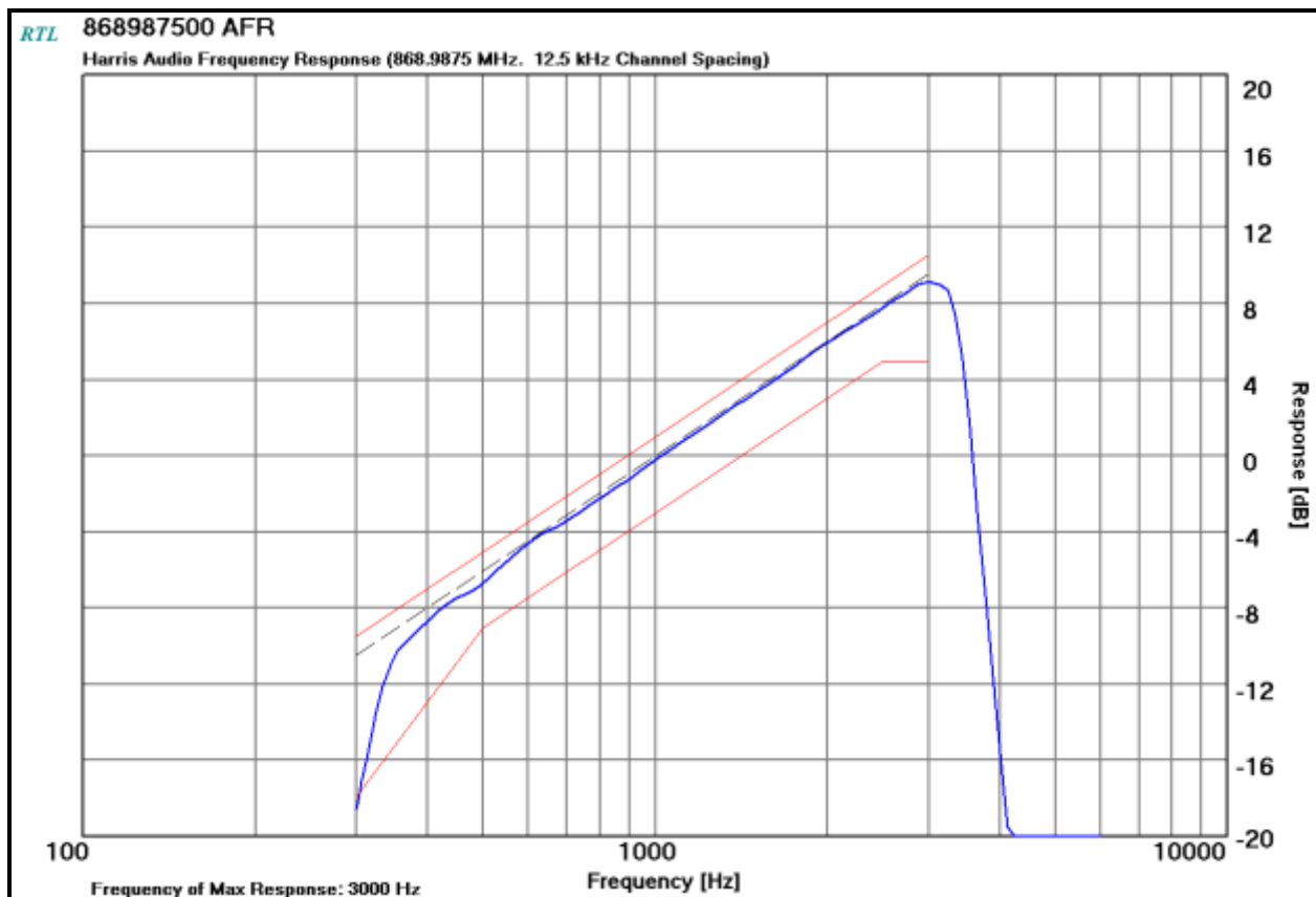
Plot 10-15: Modulation Characteristics - Audio Frequency Response – 868.9875 MHz
