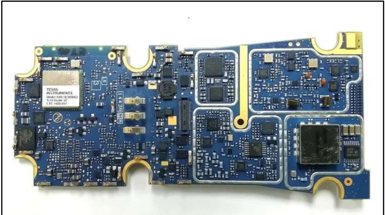
Photograph 14: Bottom without Shields
